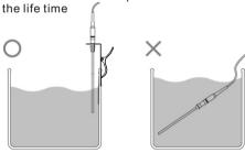
2. Suggest not to hold the probe handle while measuring high temperature. Better to use probe holder for safety.
