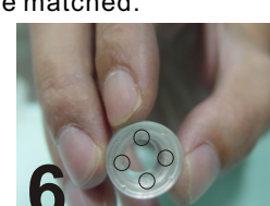
6 Find out the alignment points inside the ring of step4 semi-assembly part
