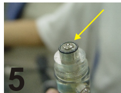
5 Put the black O-ring on the top of sensor. Make sure the O-ring is flat.
