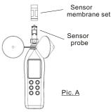
Unscrew the black globe and remove it. There is a dust free membrane to protect the humidity sensor, please remove it as well before calibration(Pic A). Reverse way to install the membrane and globe set after calibration.
