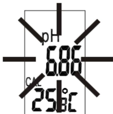
5. If the probe is damaged or the buffer is not specified as following, the primary LCD will keep flashing unless you escape by turning off the meter.
