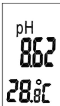
4. Press "
