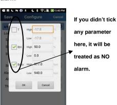
For example: Temp. is marked, High is 8  $\,^{\circ}\mathbb{C}\,$  and Low is 2  $\,^{\circ}\mathbb{C}\,$ , it means that an alarm condition will occur below 2  $\,^{\circ}\mathbb{C}\,$ , or above 8  $\,^{\circ}\mathbb{C}\,$ . The programmable alarm limit of each parameter is limited to one decimal.
