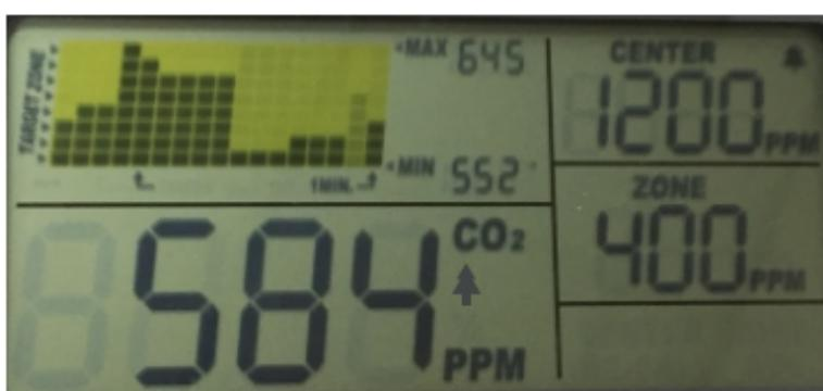
The device constantly displays current ambient CO<sub>2</sub>, set center value and set zone value.
